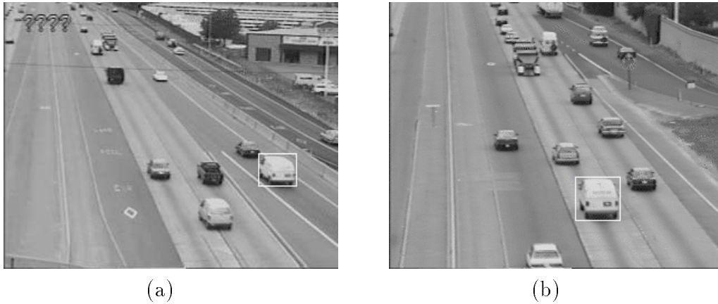
Fig. 1. Images from upstream (a) and downstream (b) surveillance cameras roughly two miles apart on Highway 99 in Sacramento, California. The boxed vehicle has been identified at both cameras.
